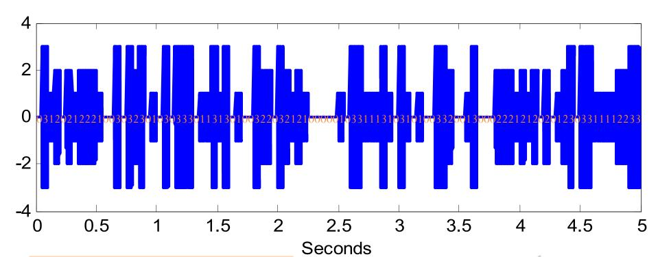
$f_c = 100 \text{ Hz}$ Symbol rate = 20 symbols per second Bit rate = 40 bps
