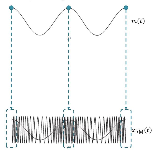
The time at which m(t) is at its maximum value corresponds to the time at which  $x_{FM}(t)$  has maximum frequency.
