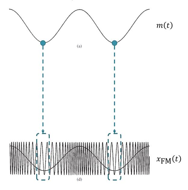
The time at which m(t) is at its minimum value corresponds to the time at which  $x_{FM}(t)$  has minimum frequency.
