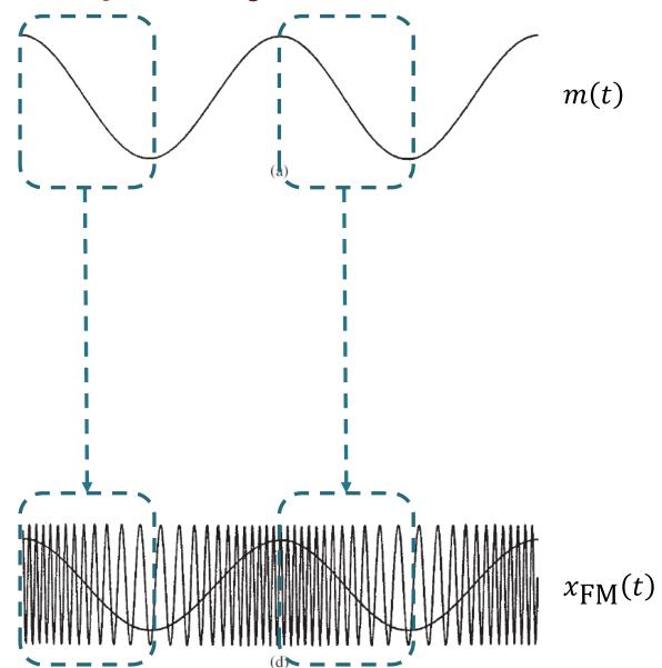
The time interval during which m(t) is decreasing corresponds to the time interval during which  $x_{FM}(t)$  has decreasing frequency.
