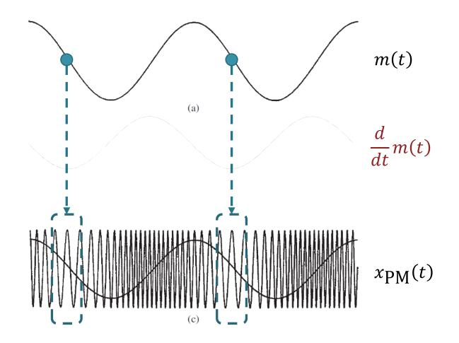
The time at which the **slope** of m(t) is at its **minimum** value corresponds to the time at which  $x_{PM}(t)$  has **minimum** frequency.
