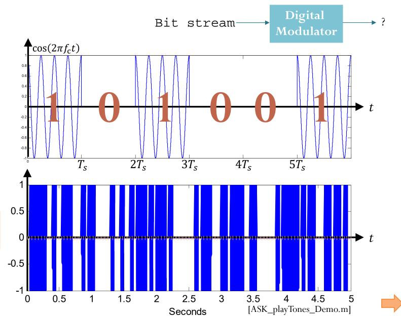
$f_c = 4 \text{ Hz}$ Bit rate = 1 bps
