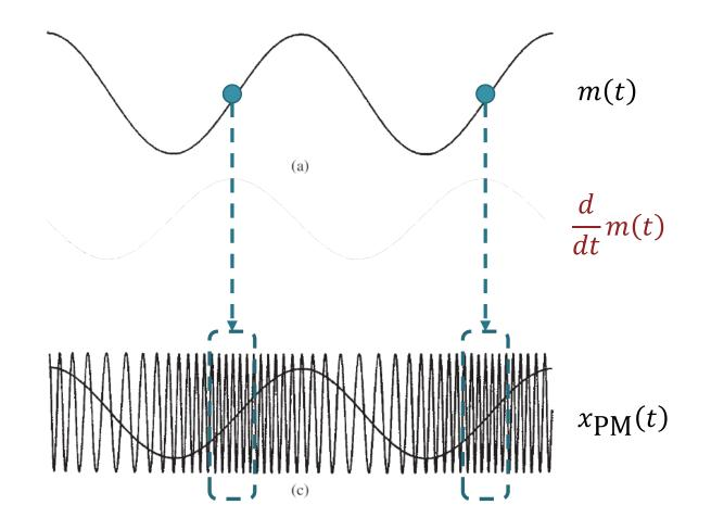
The time at which the slope of m(t) is at its maximum value corresponds to the time at which  $x_{PM}(t)$  has maximum frequency.
