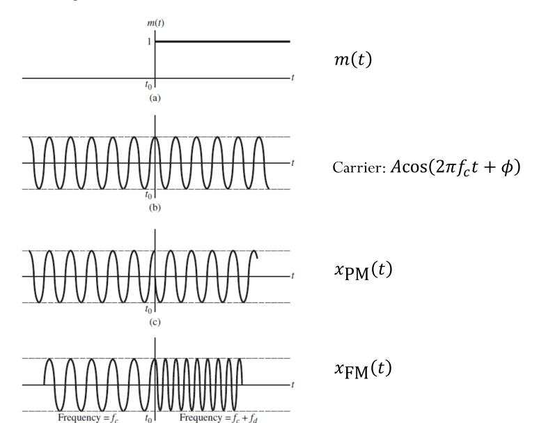
$$\left(x_{\text{PM}}(t) = A\cos\left(2\pi f_c t + \phi + k_p m(t)\right)\right)$$
