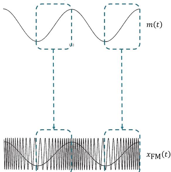
The time interval during which m(t) is increasing corresponds to the time interval during which  $x_{FM}(t)$  has increasing frequency.
