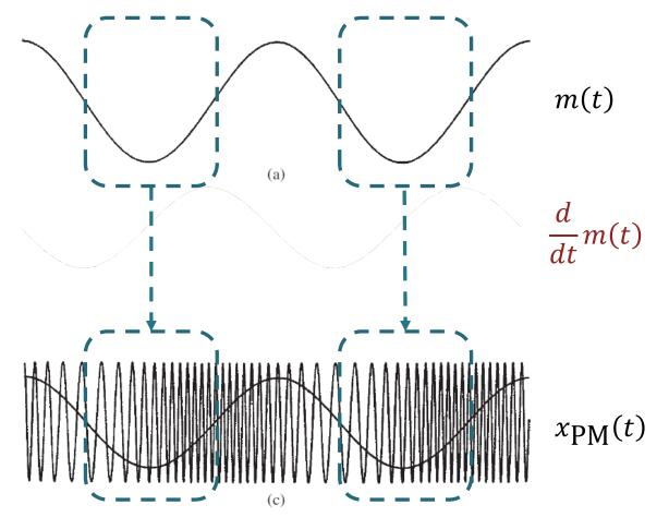
The time interval during which the slope of m(t) is increasing corresponds to the time interval during which  $x_{PM}(t)$  has increasing frequency.
